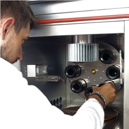
Detail of RFTO chamber, with internal light
